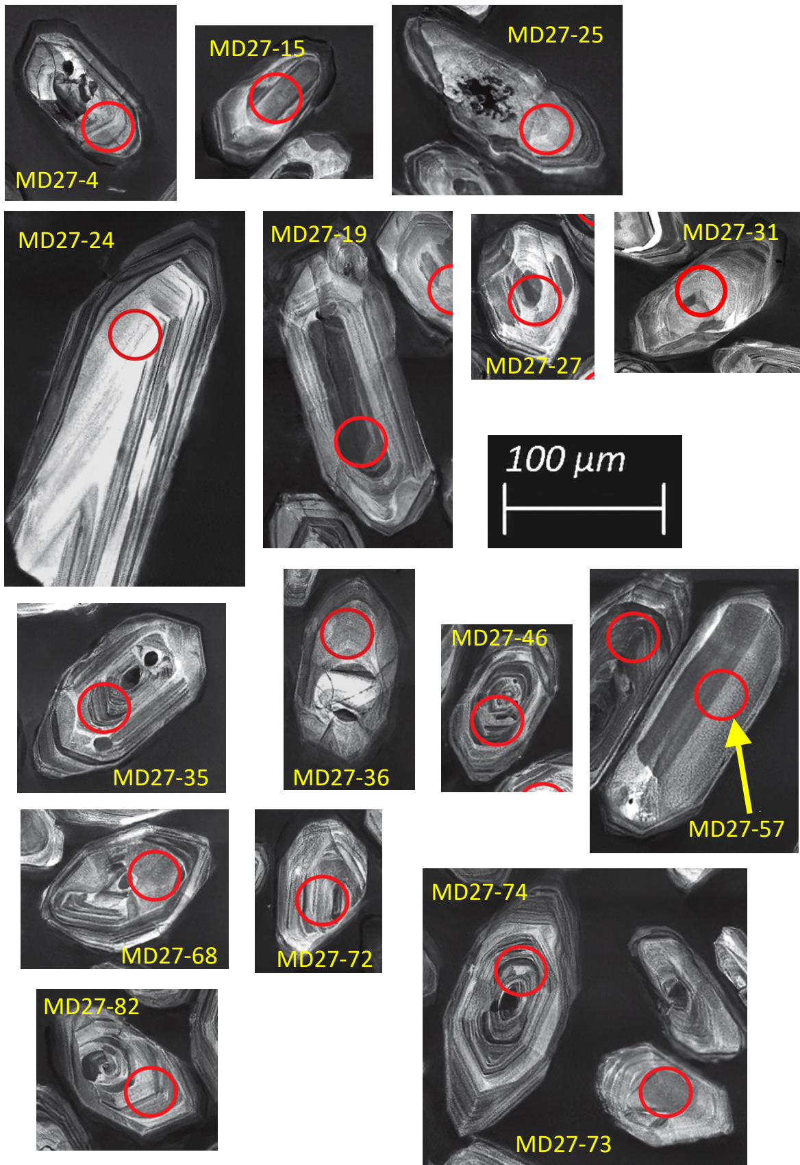
Figure A3.4. Analysed spots in zircon crystals from the Mount Disappointment Granodiorite (monzogranite), sample MD27.
